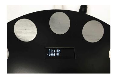
To enter this menu, scroll all the way down to the 'Looper' screen (or the Program change Pr: on earlier versions of the firmware) and then pull down and hold the rotary control for a count of three seconds and then release. You should then see this menu with Flip selected. You will be able to scroll down to the sensitivity setting and back up in the normal way.
