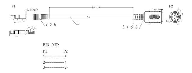
Note that it's very easy to mix up pins 4 and 5. The diagram above is looking at the user end of a \*socket\*. If looking at the pins of a \*plug\*, or when looking at the inside/solder side of a socket, the pins will be mirrored. If you're making a lead and it doesn't work right away, then it's likely that you've reversed 4 and 5. (This shouldn't cause any harm.)
