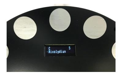
This menu displays the current scale or mode, the root note or key, and the octave.
